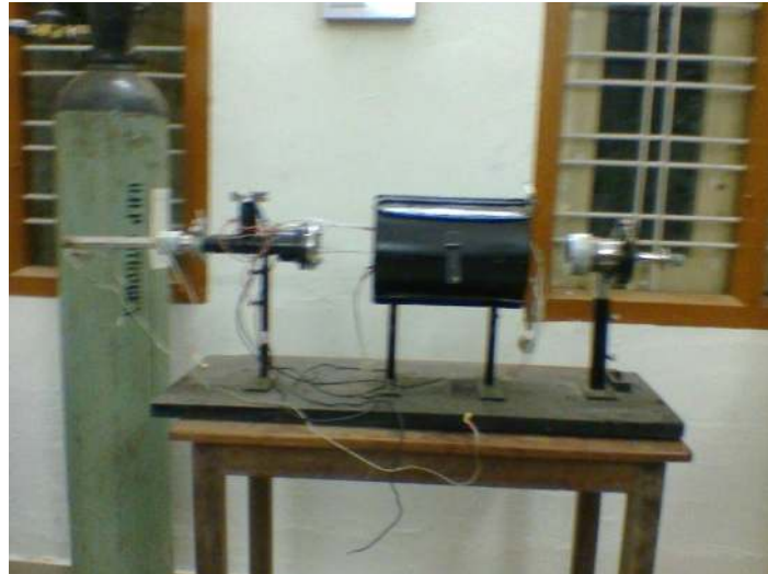
Tungsten-halogen lamp based rapid thermal annealing system
